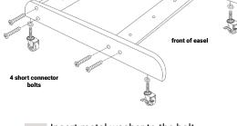
Insert metal washer to the bolt of caster. Attach caster with lock to front and caster to rear.
