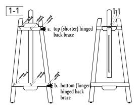
3) Attach top (See 1-1) and bottom (See 1-2) back braces to the hinged cross braces using (6) 1<sup>1</sup>/<sub>4</sub>" screws through pre-drilled pilot holes.
